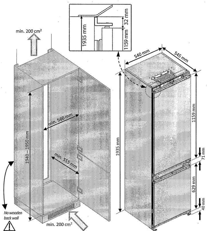
The back wall of the wooden cabinet must be left open completely to kitchen wall in order to allow sufficient air circulation to cool down the condenser unit for energy efficiency.
